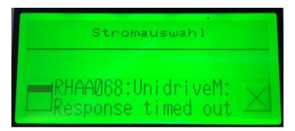
the connection between the frequency converter and the display is broken. In this case please check the connectors from the display and frequency converter.
